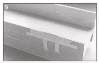
After 24 hours, remove the tape and cellophane and carefully sand the repaired area as seen in Picture R. Complete this repair by employing the Resin Sealing repair procedure.
